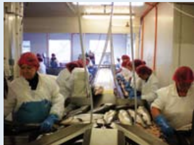
Grading and cleaning
