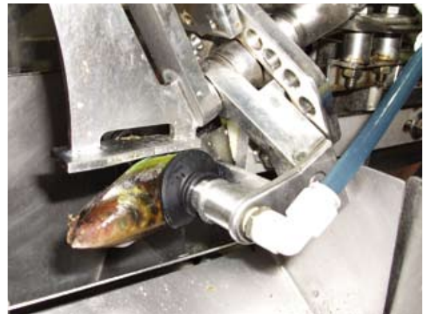
Mussel about to be opened in the automatic opening machine
