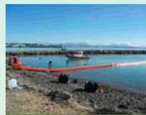
Launching of a land/sea boom in Evans Bay, Timaru Harbour, during Environment Canterbury's annual oil spill training exercise
