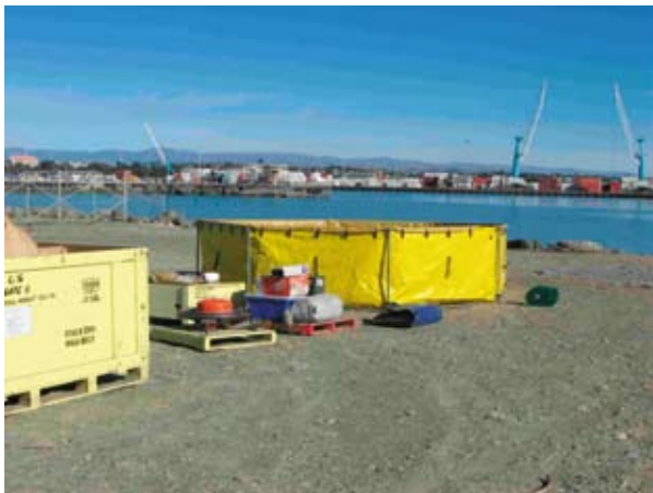
A collapsible 15-tonne oil-receiving tank used during an oil spill training exercise
