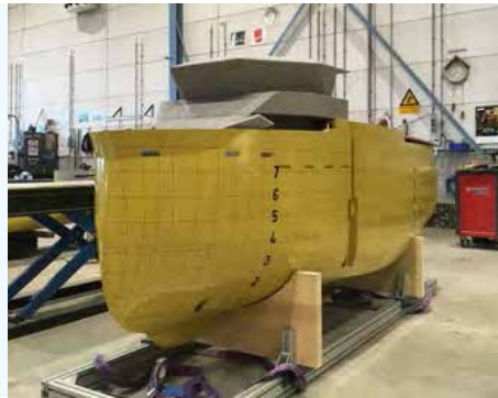
ABOVE Scale model used for tank testing
