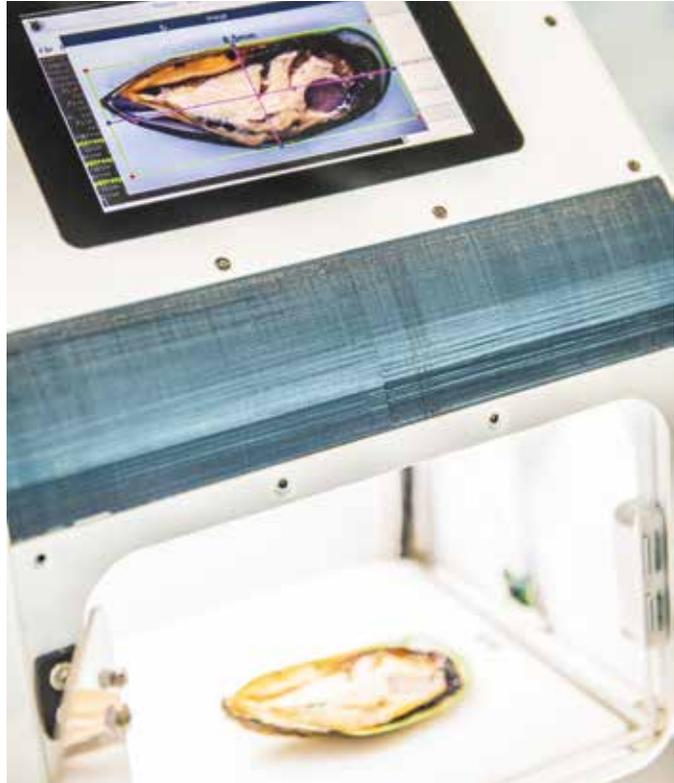
PHOTO: Sanford's mussel vision machine assessing mussel qualities using AI technology
