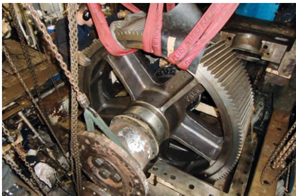
San Nanumea – main bull gear (weighing around 5 tonnes) being removed during gearbox repairs
