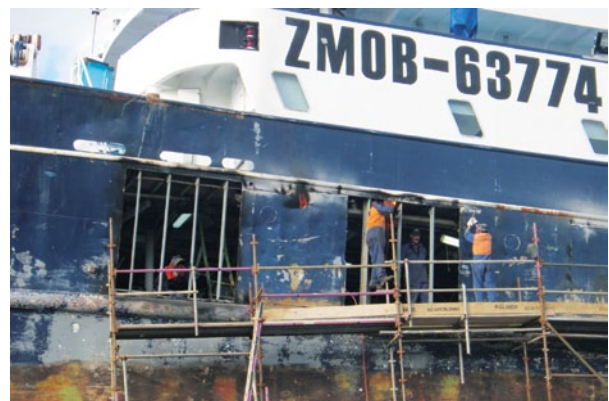
Ocean Breeze – sections of hull plate being replaced
