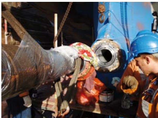
Stern shaft survey during dry-dock
