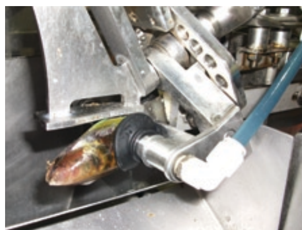
Mussel about to be opened in the automatic opening machine
