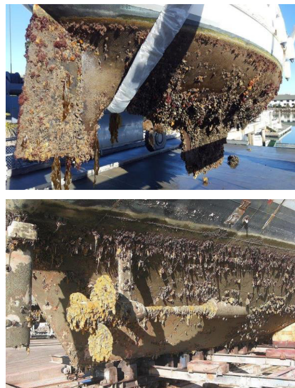
Fig. 2. When vessel hulls are not maintained, biofouling can be a significant contributor to regional and national marine pest risk
