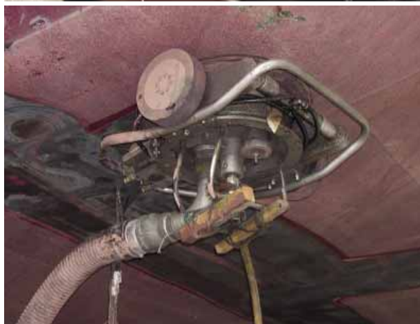
Top San Aspiring entering Timaru for the first time Middle Timaru based inshore vessel, Tengawai Bottom A "spider" remotely controlled, removing paint from San Enterprise hull. Paint flakes and water are sucked directly into a tanker
