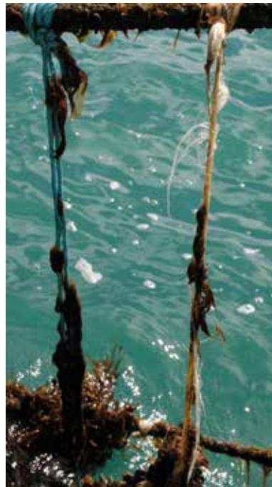
Trial comparing plastic lashing (left) with the new ECO Rope (right)
